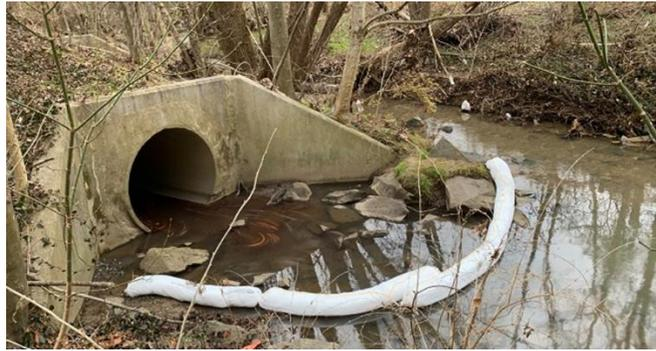
Contamination boom contains heating oil spill
